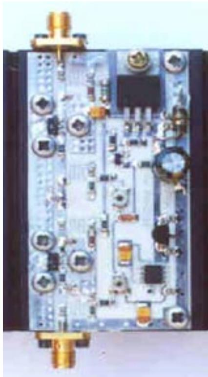
mine if better results can be obtained. One pleasing result was that the shoulders were at -38dbc that being due of course to the use of Class A type transistors which run on a +28v supply. As a matter of interest the Marconi power-measuring unit showed an output power level of around +29dbm where as all other measurements were done on the Spectrum Analyser.
