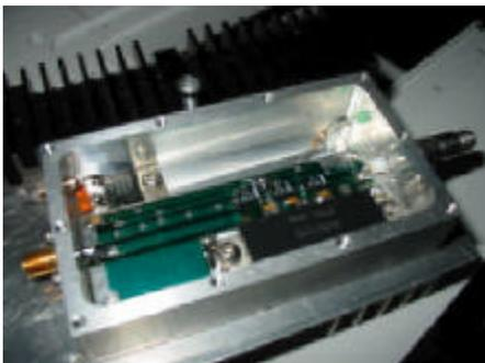
the future to combine two M67715 power modules to provide some extra output while still maintaining the shoulders at around -28dbc. It was decided not to use the M67762 power module due to poor intermod performance as is. Although I have seen some mention on the Web using this device with modifications to the bias circuit for an output power of
